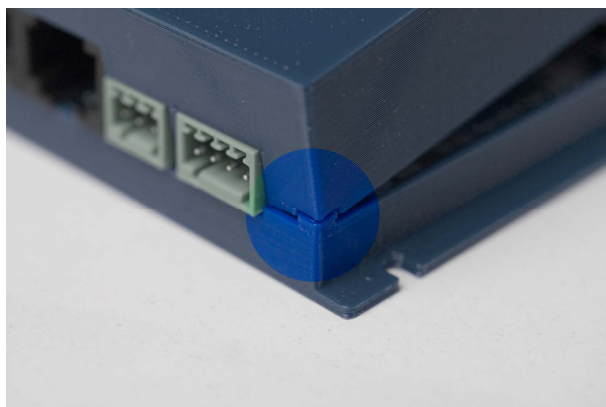
Fig 4: Closing the enclosure
